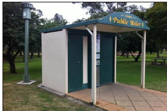
Exeloo toilet units are very robust and made from non-organic materials so they can withstand a flooding environment provided they are well secured to good foundations. There are many examples of Exeloo toilet facilities located on river banks and in flood prone areas where the water has flooded through the buildings. The building itself can normally be cleaned out with a water blaster after the flooding and put back into service but the electronic equipment often needs replacement or repair.
